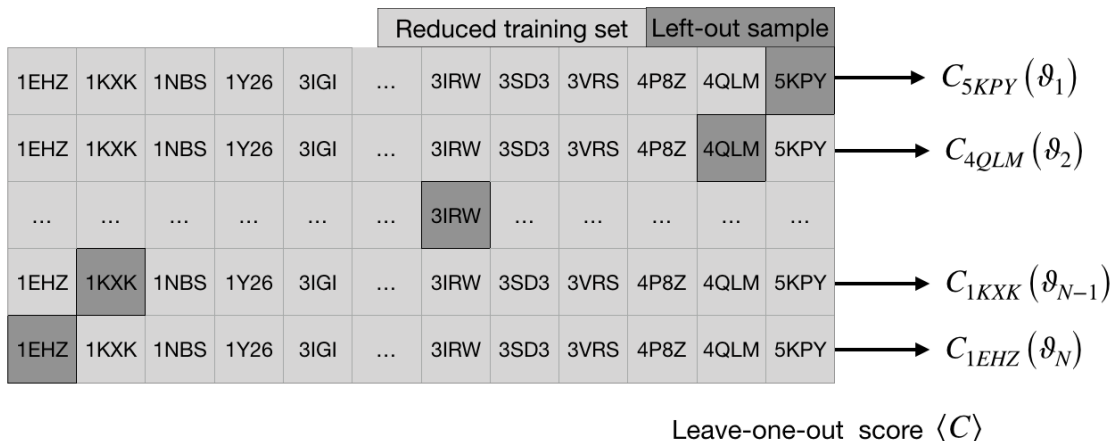
Figure 2.4: Leave-one-out test for model transferability: at iteration i , the i -th molecule is excluded from the training set of size N , and the model parameters are optimized on the reduced training set containing the other N - 1 molecules; the resulting optimal parameters \vartheta_i are used to evaluate the cost function \mathcal{C} on the left-out sample. The average of the cost function over all the estimates is used as a transferability score to rank the models and select the one with highest estimated transferability.
