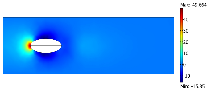
Figure 9. Pressure field of the initial shape of the bulb in plane XY (Pa).
