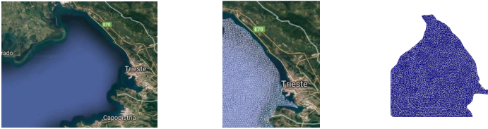
Figure 6.1: Pollutant Control . Left . Satellite images of the Gulf of Trieste. Center . Zoom of the mesh overlapping satellite images (Trieste harbour). Right . The final mesh.
