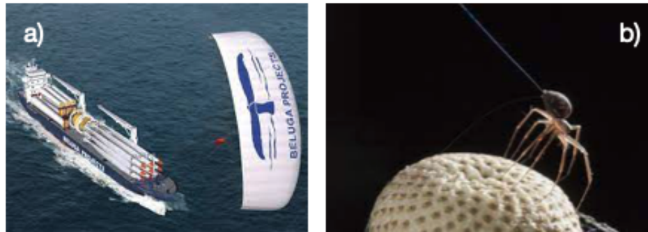
Figure 1: a) An example of application of Airborne Wind Energy technology for ship transport by the French company SkySails. The kite uses the wind to reduce the fuel consumption by the diesel engine, contributing to pull the ship across the sea. b) A spider on the verge of taking off and perform ballooning: the air can drag the silk filament, which works as sail and makes the spider become airborne.
