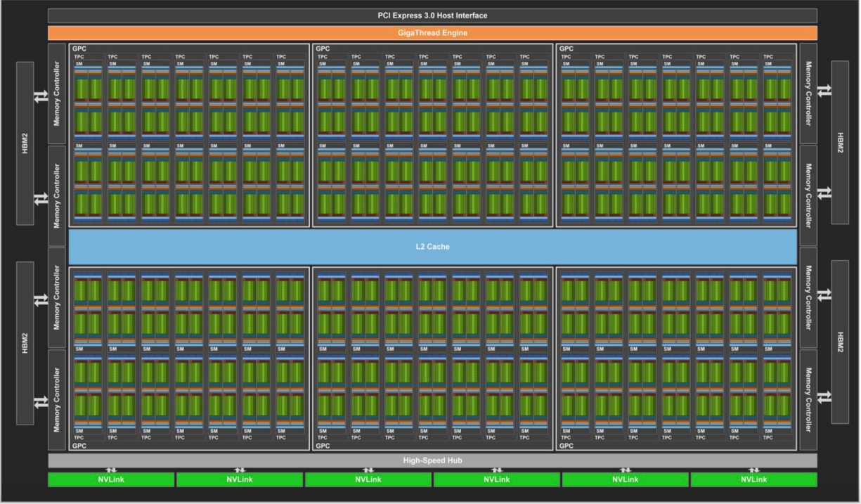
Figure 3.2: A Full NVIDIA GV100 Architecture [29].
