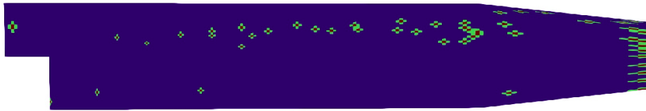
Figure 4.28: The 50 Lagrangian points are represented in red, the stencils of the cells and associated degrees of freedom needed for the evaluation of the discrete differential operators are in light-green. The discarded nodes in the evolution of the dynamics are in blue. The stencil is made by 1 layer of cells.
