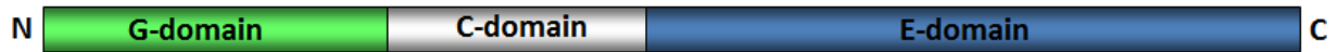
Figure 8. Gephyrin structure: splice variant P1 of gephyrin is composed of a N-terminal G-domain from residues 1 to 181, a linker domain C-domain from residues 182 to 317 and C-terminal E-domain from residues 318 to 736.
