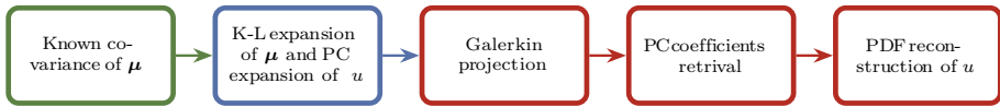
Fig. 2 Synthetic workflow diagram showing the process of computing the surrogate PDF of u by solving Equation (5) using SSFEM pipeline
