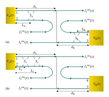
FIG. 5. Setup for the evaluation of the full HOM noise in the presence of mixing. (a) One mixing point is present on each edge. Mixing is described by the scattering matrices  $S_A$  and  $S_B$ . (b) Configuration with two mixing points (described by  $S_1$  and  $S_2$ ) on the same edge. This second setting allows us to investigate the effect of additional interferences.
