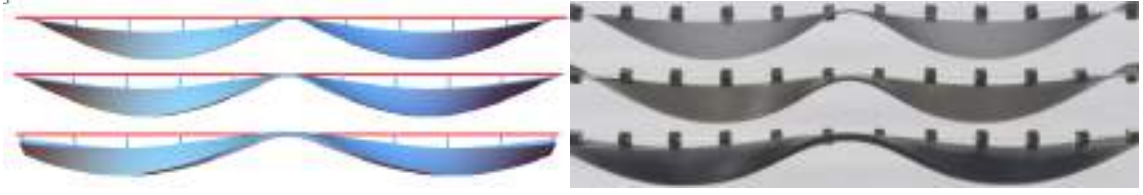
FIGURE 9. Detail of the transition zone (perversion) exhibited by a rod having L = 40 , u_2^* = 0.1 , and h/t = 20, 10, 5 (top, center, bottom). We observe that as h/t grows, the perversion is more localized.
