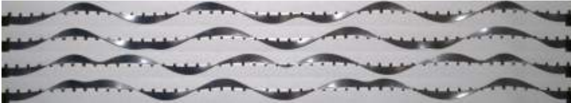
FIGURE 10. Different equilibrium configuration obtained for an experimental rod with L = 100 , h/t = 10 , u_2^* = 0.1 , exhibiting 1 (top), 2, 3, 4 (bottom) perversions.
