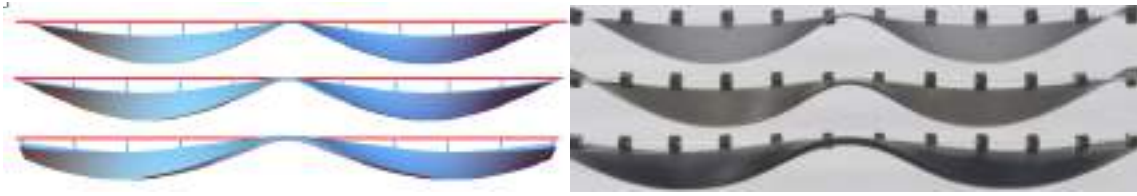
FIGURE 9. Detail of the transition zone (persion) exhibited by a rod having L = 40 , u_2^* = 0.1 , and h/t = 20, 10, 5 (top, center, bottom). We observe that as h/t grows, the persion is more localized.
