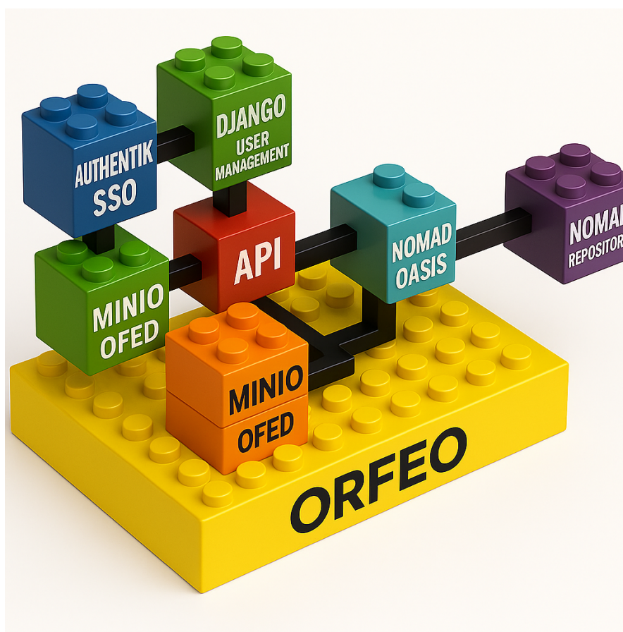
Figure 4.2: Architecture of the LAME data management system: from user authentication to data storage in MinIO, registration in ORFEO, and publication to NOMAD Oasis. The system components are represented as interlocking LEGO blocks to emphasize modularity and integration.
