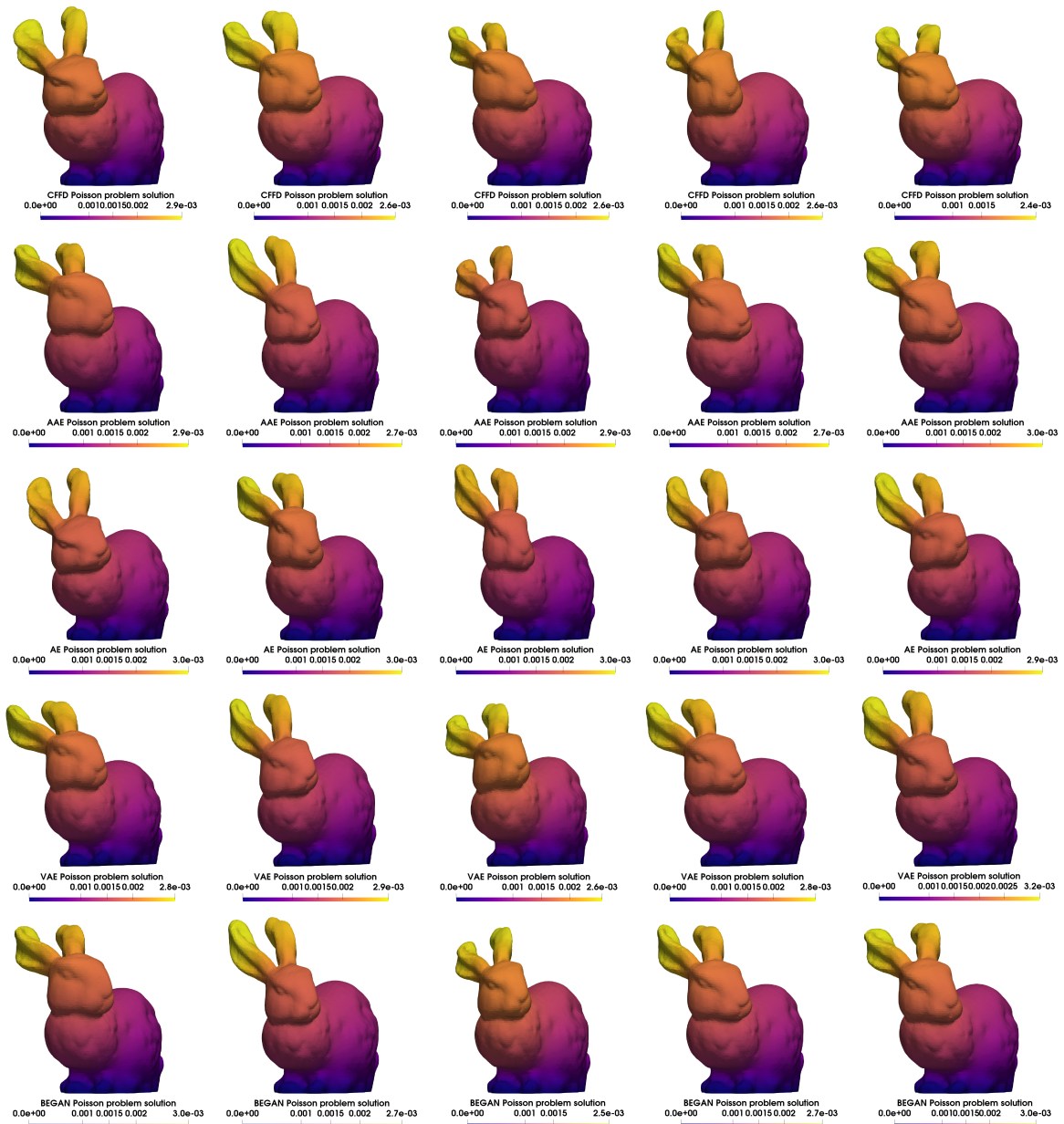
Fig. 4.5 SB . Some geometrical deformations of the Stanford bunny are shown: the first row refers to constrained cFFD of section 4.2.2, the second to the adversarial autoencoder of paragraph 4.3.1, the third to the simple autoencoder of paragraph 4.3.1, the fourth to the beta variational autoencoder of paragraph 4.3.1 and the last to the boundary equilibrium generative adversarial networks of paragraph 4.3.1. All the generative models implement the linear constraints enforcing layer of section 4.3 to preserve the position of the barycenter.
