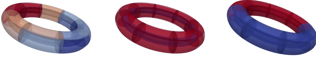
Fig. 5.4 MS . Left : FOM computational domain partitioned in K = 4 subdomains inside deal.II. Center : MS1 , DD-ROM repartitioning of the computational subdomain k = 2 with the cellwise variance indicator I_{\text{var}} , definition 7: 20% of the cells belong to the low variance part, represented in blue inside the torus, and the other 80% belong to the high variance part, represented in red. Right : MS2 , DD-ROM repartitioning with variance indicator P_l = 50\% . The computational domain is exactly split at the interfaces that separate the subdomains \{x < 0\} \cap \Omega and \mu = \sigma = 2 in which the parameters \mu and \sigma are constant.
