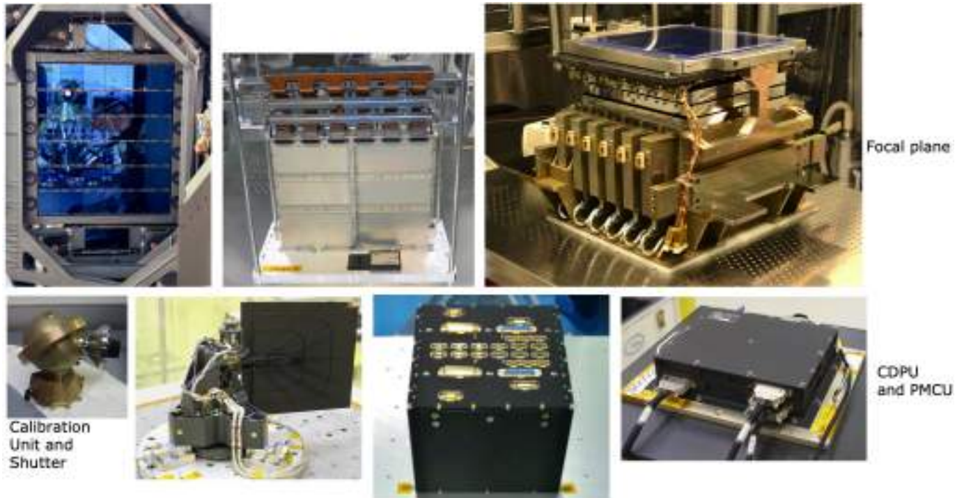
Fig. 9. Constituents of VIS. Top: The VIS focal plane showing (from left to right) the array of 36 close-butt CCDs within their SiC structure, as integrated on the PLM; a ‘slice’ of six CCDs with a pair of ROEs to control them and digitise the signals; and the integrated focal plane with a protective cover for the CCDs (six power supplies for each ROE can be seen on the left of the structure with the other six out of view behind it). Bottom: From left to right: the CU used for providing a flat illumination of the focal plane at six different wavelengths; the shutter; the Control and Data Processing Unit, which controls the instrument, sequences the 144 channels of data from the 36 CCDs, compresses the image, and communicates with the spacecraft; and the Power and Mechanism Control Unit, which drives the shutter and the CU. All of these have redundant halves except for the multiplexers on the CDPU to the 12 ROEs.
