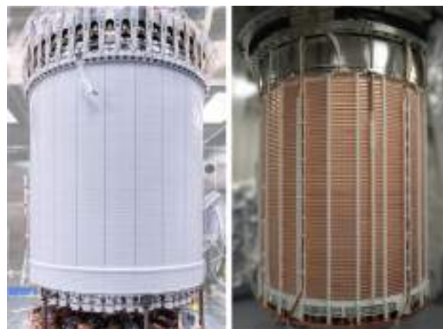
Fig. 6 The LZ (left) and XENONnT (right) LXe-TPCs containing 7-tonnes and 5.9-tonnes of liquid xenon in the active detector volume, respectively. Both TPCs have a drift length of around 1.5 m, while the diameter of the sensitive target is 1.5 m in LZ and 1.3 m in XENONnT
