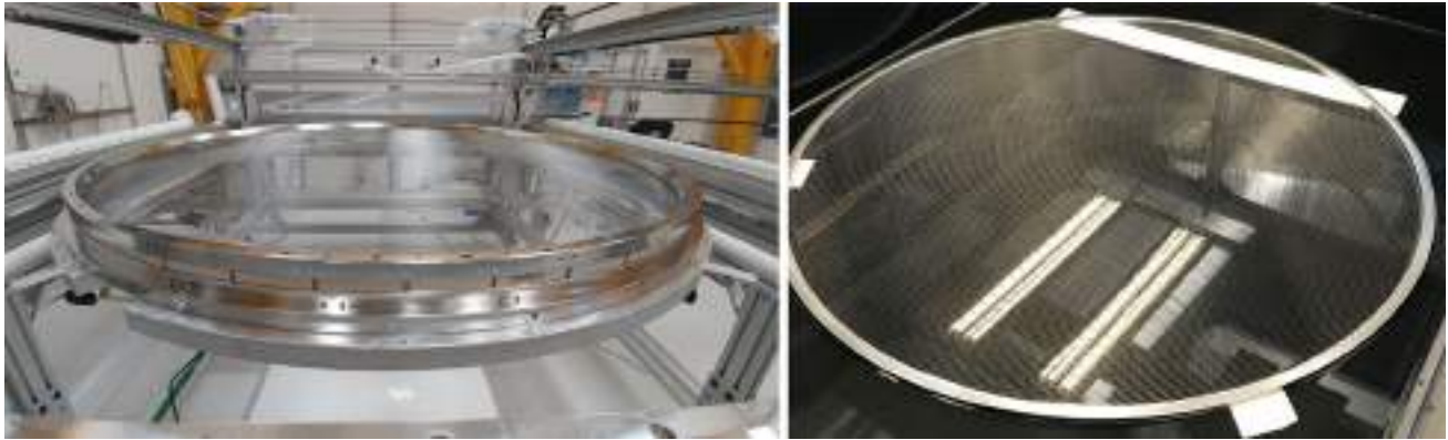
Fig. 8 A finished LZ grid with crossed wires on the custom loom (left) and a XENONnT electrode with parallel wires (right)
