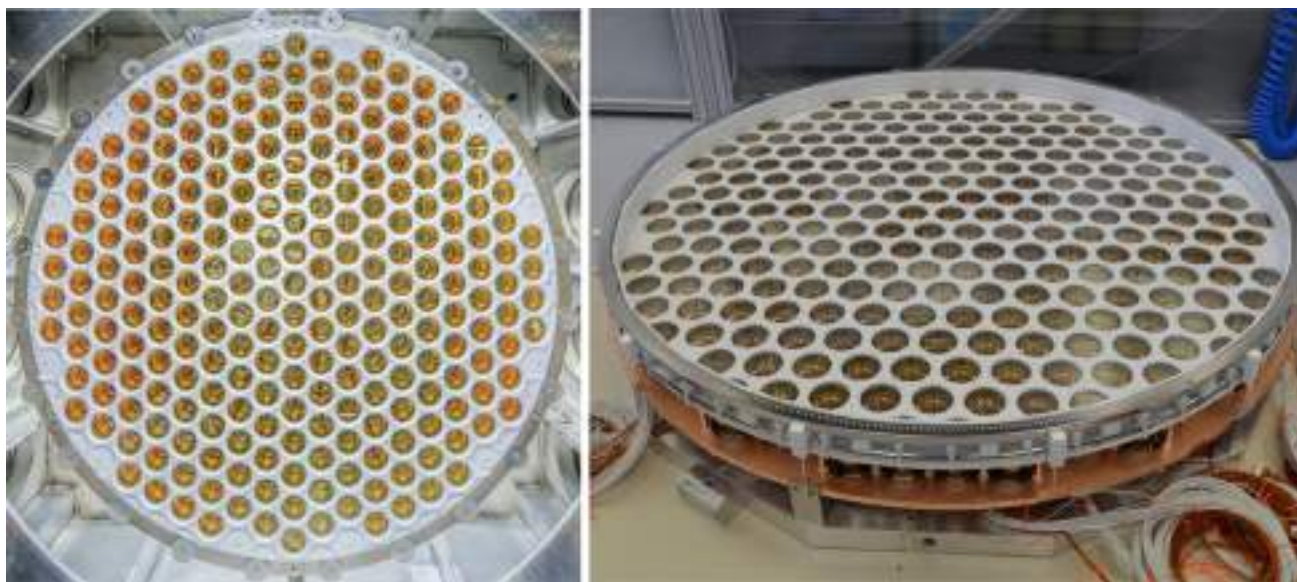
Fig. 9 The LZ bottom (left) and XENONnT top (right) PMT arrays. Each experiment has 494 R11410 Hamamatsu PMTs installed
