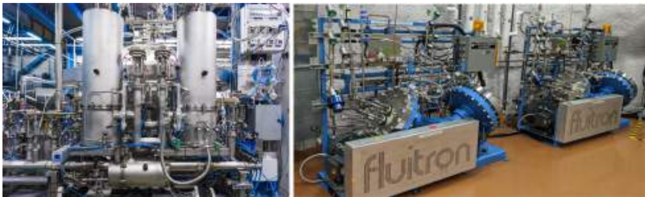
Fig. 12 Left: the XENONnT liquid purification system currently installed at LNGS. Right: the high-purity high-pressure Fluitron gas compressors used for LZ circulation and recovery
