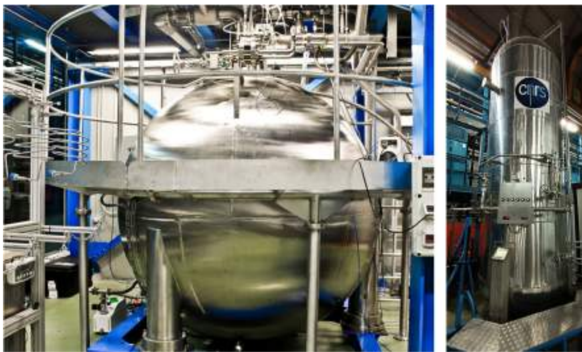
Fig. 11 The ReStoX I (left, 7.6 tonne capacity) and ReStoX II (right, 10 tonne capacity) on-site cryogenic storage systems for XENONnT have demonstrated high-purity storage of xenon gas and liquid [104]
