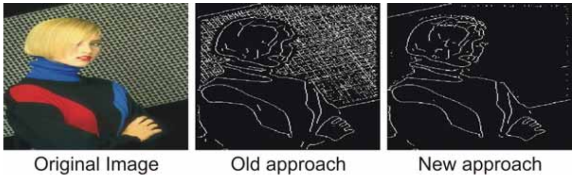
Figure 2.5 Comparison of old and new approach for Edge detection
