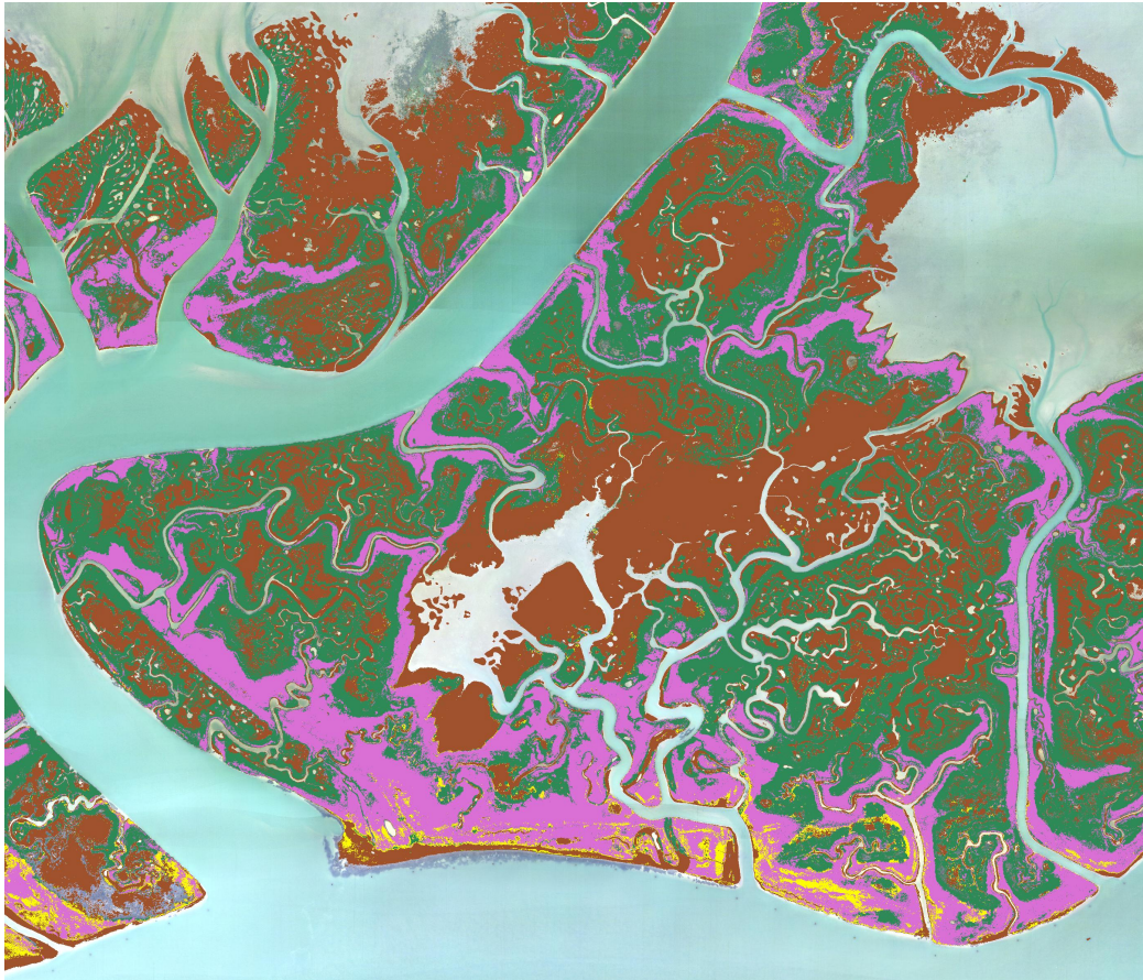
Figure 1.10: Same image as before, but with the classification of the vegetation superimposed. Legend: maroon: soil, green: spartina maritima ; yellow: sarcocornia fruticosa , pink: limonium narbonense . Courtesy of TIDE project.
