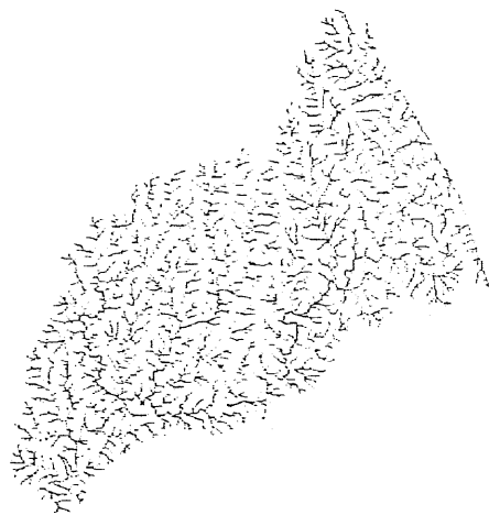
Figure 2.3: A river network image. The colors in this image blue, green, yellow, orange, red, and black correspond to streams of different Stralher orders [1, 2]. Stralher ordering system is the most common classification scheme of the hierarchical branching structure of river networks used in hydro-geomorphology.
