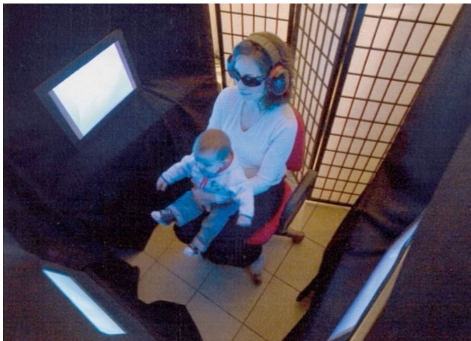
Figure 8: The experimental setup of the head-turn preference paradigm used in all the infant studies reported in the thesis. The picture is taken from the top of the left corner of the testing booth. The three monitors at the center and at the sides are in light blue just to show their arrangement inside the booth. During the experiment, they would otherwise be in black, with only exception of the colored visual attractor (see Procedure). The camera recording the infant's looking behavior is located above the central monitor; it is not visible from the picture as it is hidden behind the black curtain.
