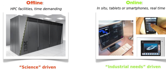
Figure 2: The main idea behind reduced order model: offline-online splitting of computational phases.
