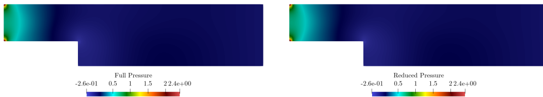
Figure 6: Comparison between pressure solutions: high fidelity on the left, reduced order on the right.
