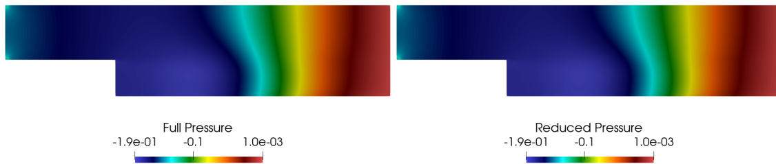
Figure 25: Comparison between pressure solutions: high fidelity on the left, reduced order on the right.
