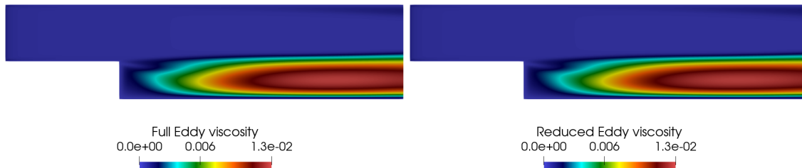
Figure 27: Comparison between eddy viscosity solutions: high fidelity on the left, reduced order on the right.
