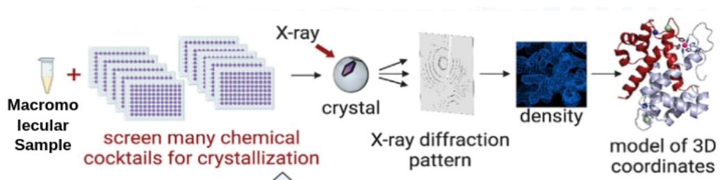
Figure 2.1: Experimental pipeline to produce structural information of macromolecules based on XRD method [6]
