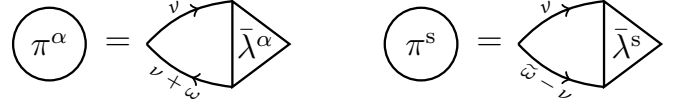
FIG. 11. Relation between the polarization and the right-sided Hedin vertex \bar{\lambda} (similar relations hold for the left-sided \lambda by attaching legs from the right). (Left) Particle-hole channels. (Right) Singlet-particle-particle channel.
